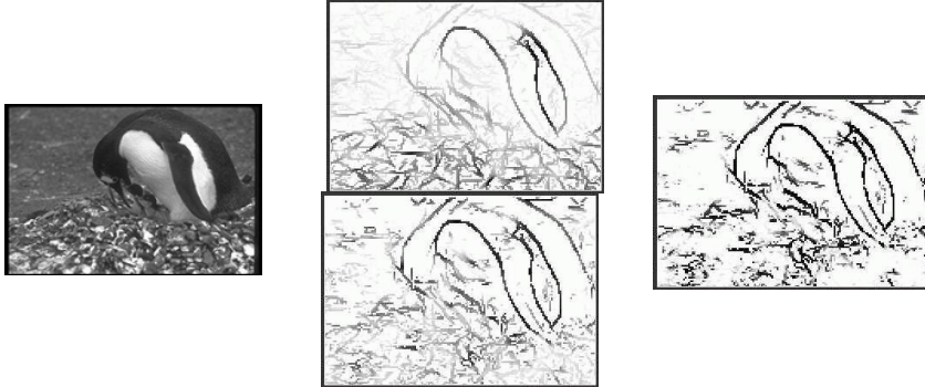
Figure 10. Gating the contour cue. Left: original image. Top: oriented energy after nonmaximal suppression, OE^* . Bottom: 1 - p_{texture} . Right: p_B , the product of 1 - p_{texture} and p_{con} = 1 - \exp(-OE^*/\sigma_{IC}) . Note that this can be thought of as a “soft” edge detector which has been modified to no longer fire on texture regions.
